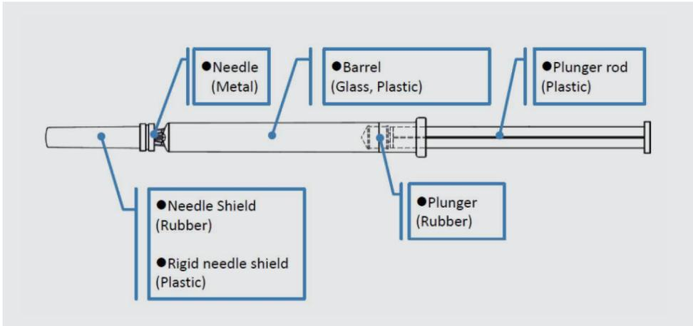
Figure 3: Multiple contact parts content in a prefilled syringe.
